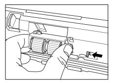
**4.** Push the roller lock lever towards the back of the scanner to lock the roller unit in place.
