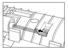
**3.** Push the roller lock lever towards the back of the scanner to lock the retard roller in place.
