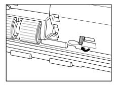
**3.** Supporting the roller unit with your hand, slide the roller lock lever to the right.
