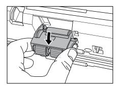
**5.** First detach the right side of the roller unit (1), and then remove the roller unit (2).
