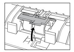
**3.** Move the roller lock lever upward (1), and then slide it to the right (2).
