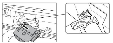
**2.** Insert the protrusion of the roller unit into the groove in the scanner, and then lift the roller unit.
